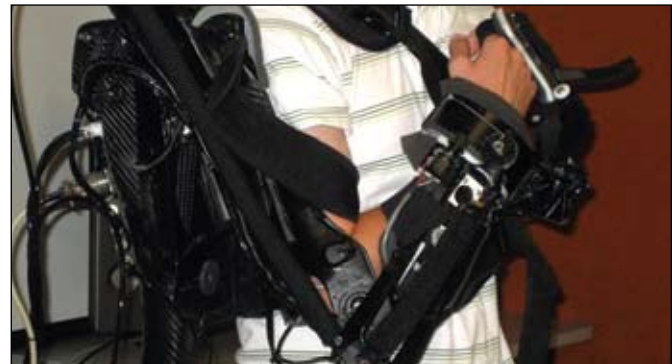
Figure 2. Robotic Upper Extremity Repetitive Trainer.
