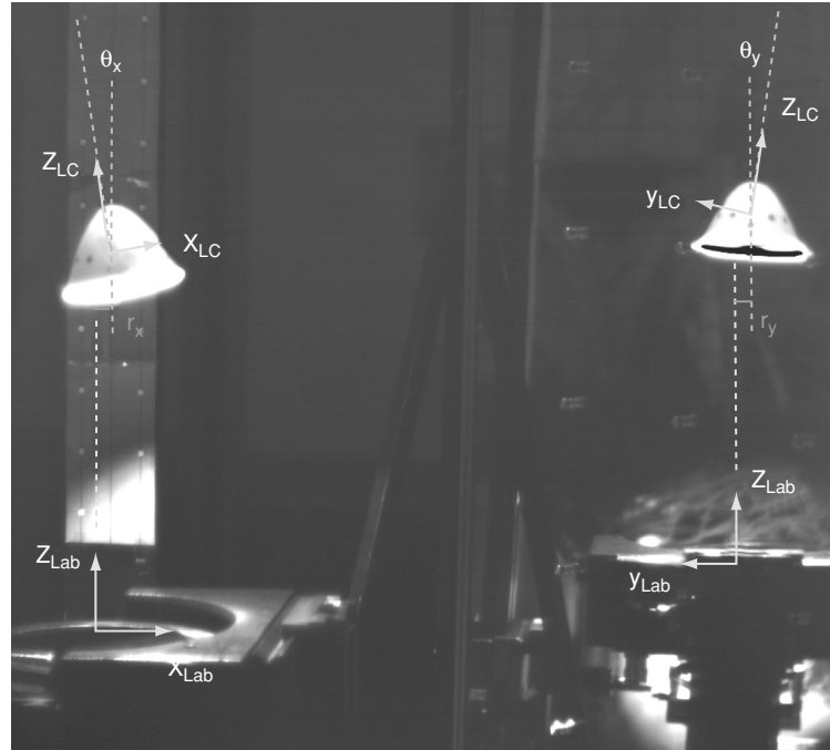
Figure 1. Test range for free flight experiments with a laser-driven thruster. This frame is taken from a high speed recording and shows recombination light from laser induced plasma. The laboratory system is denoted with an index 'Lab', whereas 'LC' refers to the coordinate system of the lightcraft. Inclination angle and lateral offset are indicated with respect to the plane of observation. In this example, r_x , \theta_x , \theta_y are positive, r_y is negative.
