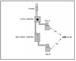
Figure 3. The measuring diagram
