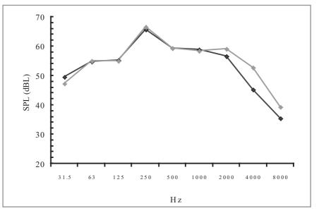
Figure 4. 1/1 octave band analysi of sound pressure level for study fans
