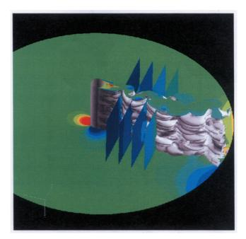
Figure 14. CFD computation of the unsteady flow in the wake of a cylinder. Isovorticity surfaces are shown and in the plane perpendicular to the cylinder are shown pressure contours. From Madsen<sup>8</sup>.
