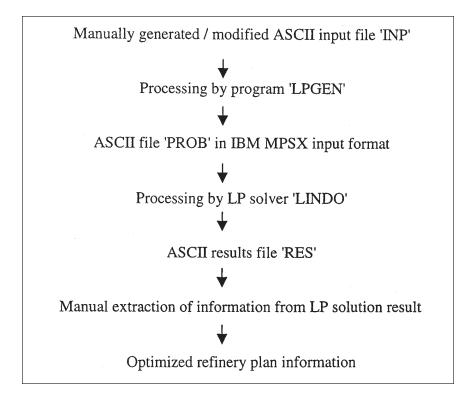
Figure 2. Flowchart for formulating and solving the LP model.
