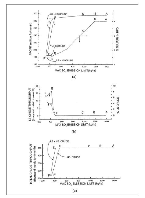
Figure 3. Variations of profit, % sulfur in RFO, LS crude throughput, and total crude throughput with maximum  $SO_2$  emission limit with free crude mix and only HS crude processing.
