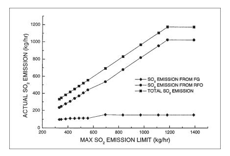
Figure 5. Contributions of SO<sub>2</sub> emissions from fuel gas and refinery fuel oil with free crude mix.
