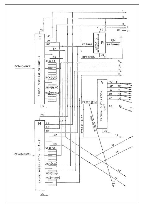
Figure 1. Schematic diagram of various units and streams of the refinery under study (cont'd.).
