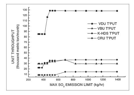
Figure 4. Variations of throughputs of secondary processing units with maximum  $SO_2$  emission limit with free crude mix.
