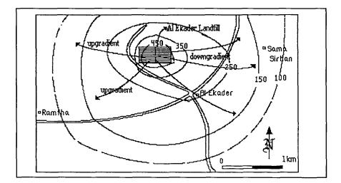
Figure 9. Leakage of leachate from AI Ekader landfill.
